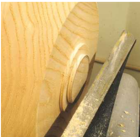
▲ Pic.7 A paring tool could be used as they need only be about 5mm deep. If you don't want to lose bowl thickness then glue a sacrificial scrap wood block on the base and turn the spigot on that
